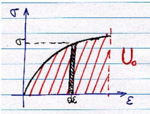
Figure 3: Strain energy density
