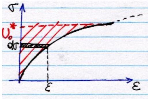
Figure 4: Complementary strain energy density
