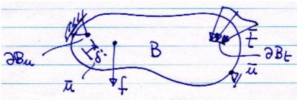
Figure 1: Schematic of generic problem in linear elasticity
