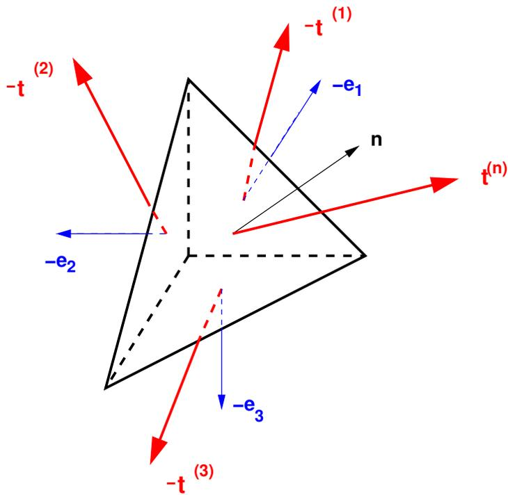
Figure 3: Cauchy's tetrahedron representing the equilibrium of a tetrahedron shrinking to a point
