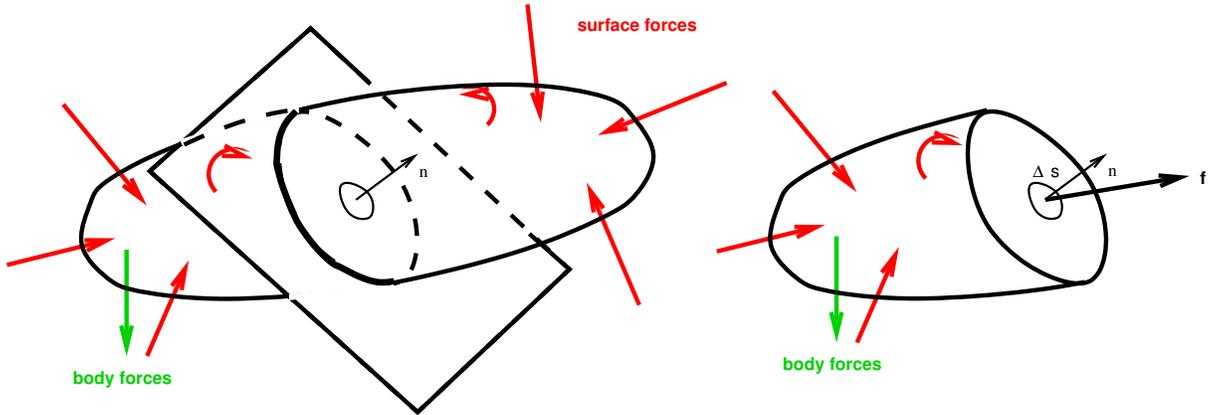
Figure 1: Surface force  $\mathbf{f}$  on area  $\Delta S$  of the cross section by plane whose normal is  $\mathbf{n}$
