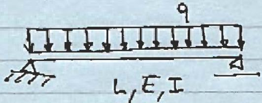
$$\Pi(u_3) = \frac{1}{2} \int_0^L EI \left( \frac{d^2 u_3}{dx_1^2} \right)^2 dx_1 + \int_0^L q(x_1) u_3(x_1) dx_1$$
