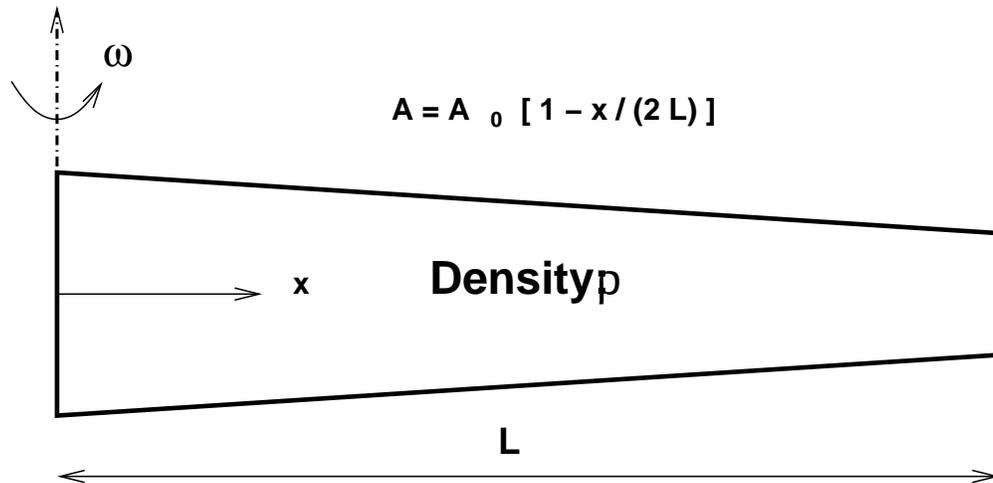
The structure of the figure is made of an elastic material with Young's Modulus  $E$ , and mass density  $\rho$  and rotates at an angular velocity  $\omega$ . (Questions start on the next page)
