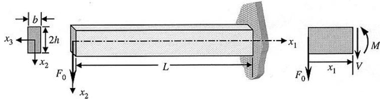
3. For the cantilever beam loaded with a point load at the free end (see figure), the bending moment  $M_3$  about the  $x_3$ -axis is given by  $M_3 = -F_0x_1$ . The bending stress  $\sigma_{11}$  is given by:
