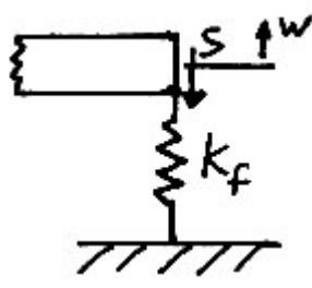
$$\left\{ \begin{array}{l} M = EI \frac{d^2w}{dx^2} = 0 \\ S = \frac{d}{dx} \left( EI \frac{d^2w}{dx^2} \right) = k_f w \end{array} \right.$$
