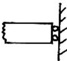
$$\left. \begin{array}{l} S = \frac{d}{dx} \left( EI \frac{d^2 w}{dx^2} \right) = 0 \\ \frac{dw}{dx} = 0 \end{array} \right\}$$
