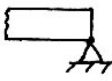
$$\left. \begin{array}{l} w = 0 \\ M = EI \frac{d^2 w}{dx^2} = 0 \end{array} \right\}$$
