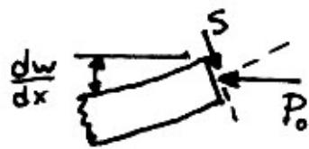
$$\left\{ \begin{array}{l} M = EI \frac{d^2w}{dx^2} = 0 \\ S = \frac{d}{dx} \left( EI \frac{d^2w}{dx^2} \right) = -P_0 \frac{dw}{dx} \end{array} \right.$$
