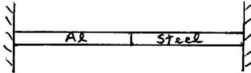
Total deformation is zero, but there will be nonzero total strain in the aluminum and steel
