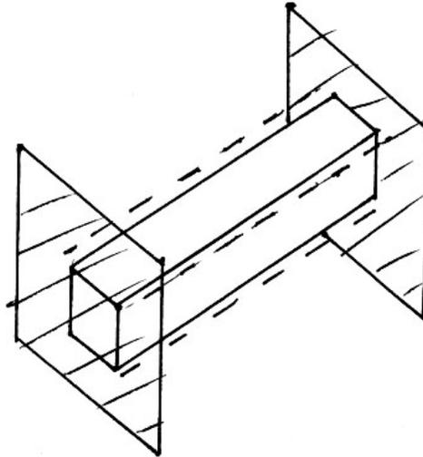
Then, as it is heated, the rod cannot lengthen. The thermal strain is the same as in the previous case but now the total strain is zero (i.e., no physical deformation).
