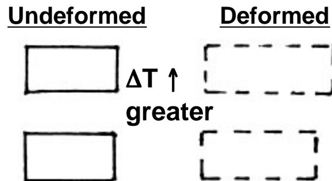
These two must deform the same longitudinally, so there must be stresses present to compress the top piece and elongate the bottom piece
