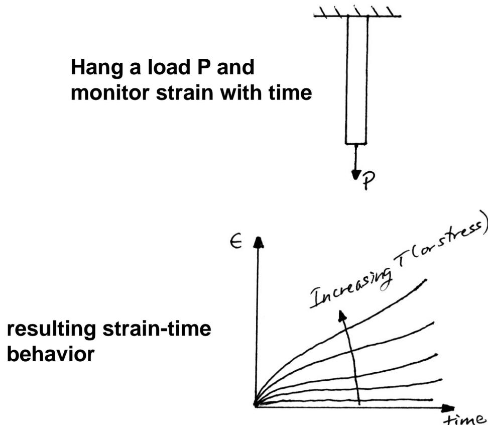
This keeps aluminum from being used in supersonic aircraft in critical areas for aerodynamic heating.
