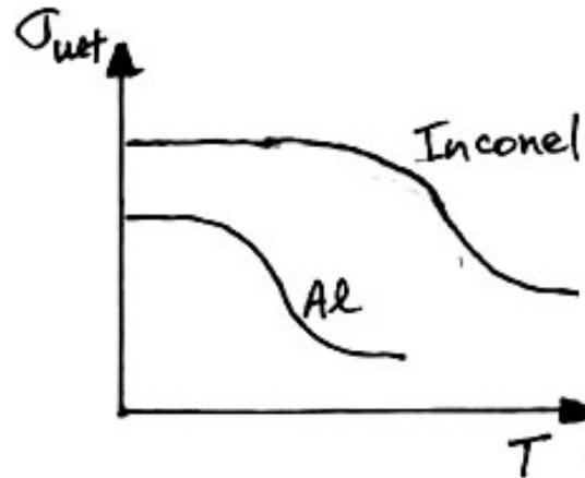
**Figure 9.11** Representation of change in stress-strain behavior with temperature
