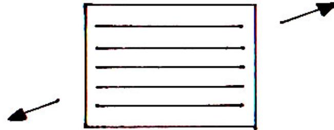
Shears with regard to loading axis but still no inherent shear/extension coupling
