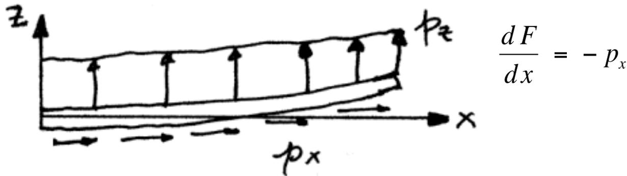
This considers only static loads. Must add the inertial load(s). Since the concern is in the z-displacement ( $w$ ):
