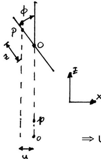
$$\Rightarrow u = -z \sin \phi \quad \text{Note direction of } u \text{ relative to } +x \text{ direction}$$
