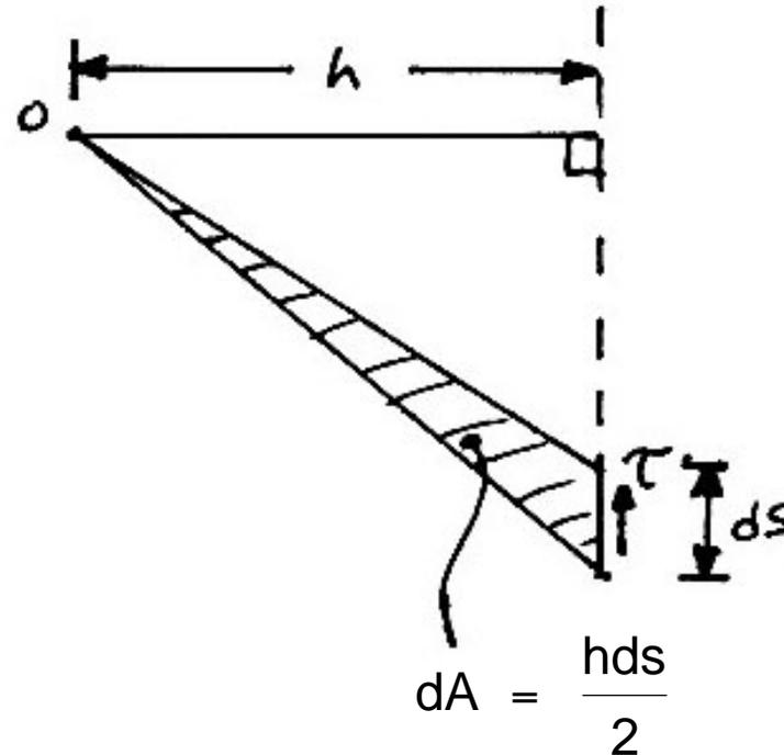
$$\left( \frac{\text{height} \times \text{base}}{2} \right) = \text{Area of Triangle}$$
