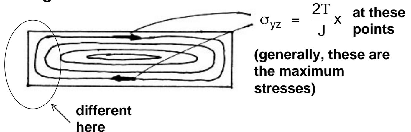
Need formulae to correct for “finite” size dependent on ratio  $b/h$ .
