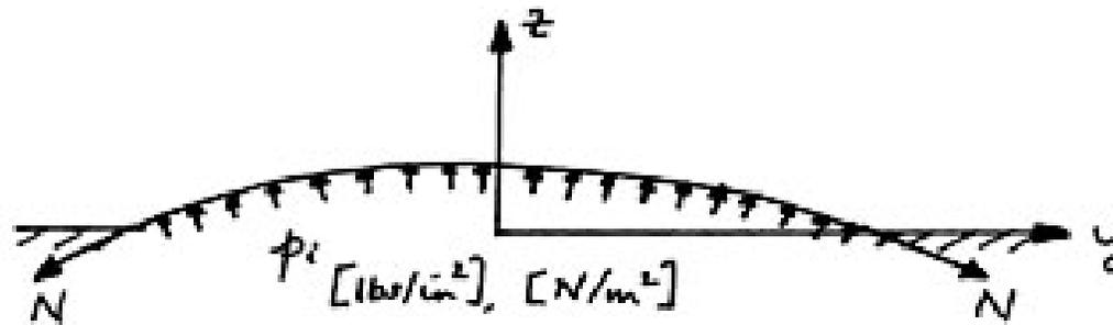
Assume: lateral displacements ( $w$ ) are small such that no appreciable changes in  $N$  occur.
