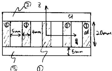
As in problem #6, the modulus-weighted centroid is at the center of the cross-section due to symmetry.
