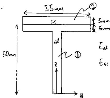
First, we need to find the modulus-weighted centroid of cross-section.
