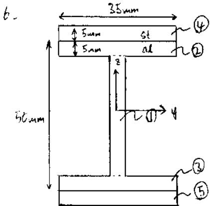
Since this cross-section is symmetric about the  $y$ -axis, the modulus-weighted centroid coincides with the "regular" centroid and is located at the center of cross-section.
