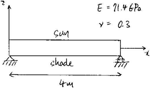
$$\alpha = 7.2 \mu\text{E}/^\circ\text{C}$$
