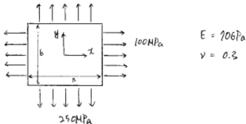
a) To construct a solution for this configuration, we need to refer to the Airy stress function sheet. From this sheet, we can see that the biaxial tension state of the current problem can be described by the superposition of uniaxial tension problems.
