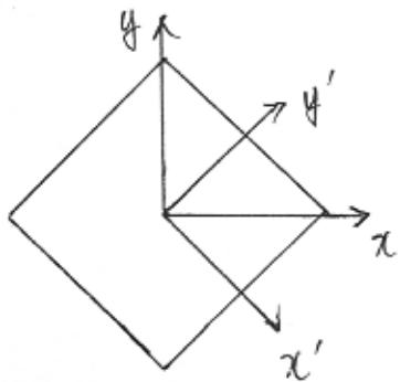
$$\left. \begin{aligned} I_{y'} &= \frac{1}{12} a^4 \\ I_{x'} &= \frac{1}{12} a^4 \\ I_{x'y'} &= 0 \end{aligned} \right\}$$
