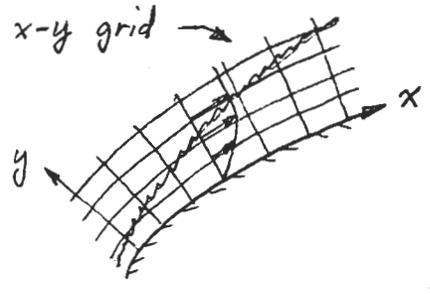
In general, the TSL will increase in thickness downstream, making a finite-difference solution on a fixed x-y grid awkward.
