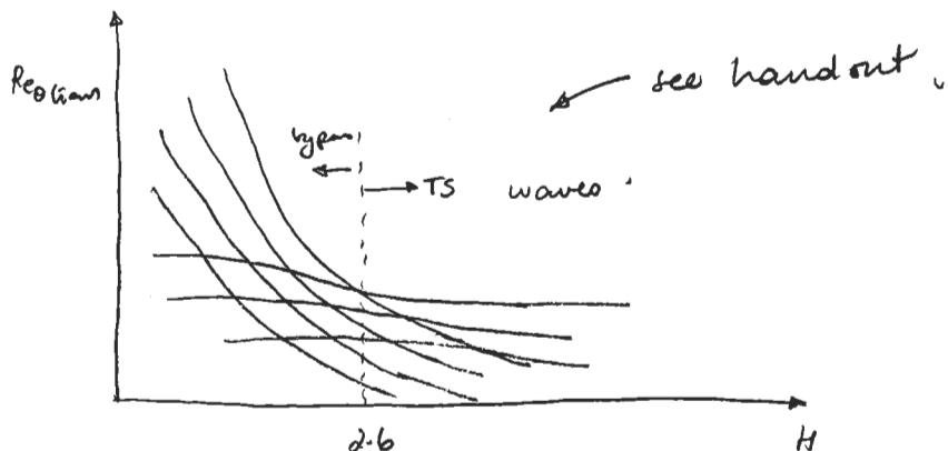
Bypass mechanism more likely to cause transition in favorable pressure gradient  $H < 2.6$
