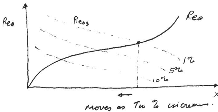
The SGS criterion is much less affected by pressure gradient than TS wave mechanism. (Transition on turbine blades with accelerating flow).
