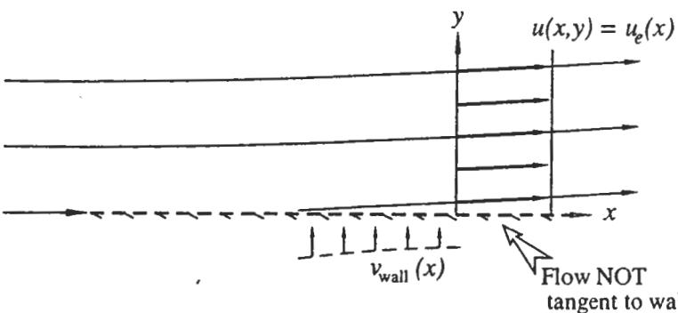
$\Rightarrow \underline{v_{wall} = \frac{d}{dx} (u_e \delta^*)}$
