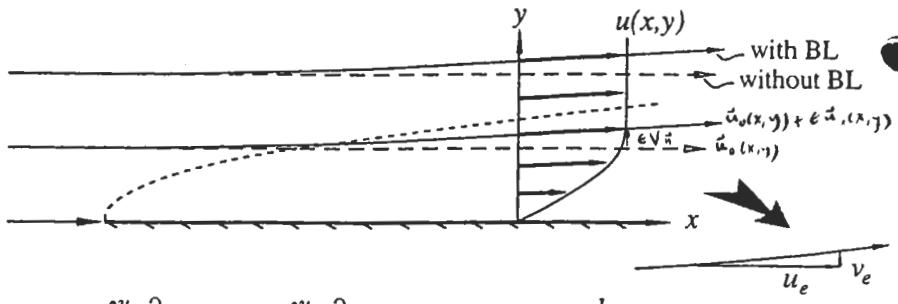
$$\begin{aligned} v(x, y_e) \equiv v_e(x) &= \int_0^{y_e} \frac{\partial v}{\partial y} dy = - \int_0^{y_e} \frac{\partial u}{\partial x} dy = \int_0^{y_e} \frac{\partial}{\partial x} (u_e - u) dy - y_e \frac{du_e}{dx} \\ &= \frac{d}{dx} \left[ u_e \int_0^{y_e} \left( 1 - \frac{u}{u_e} \right) dy \right] - y_e \frac{du_e}{dx} \end{aligned}$$
