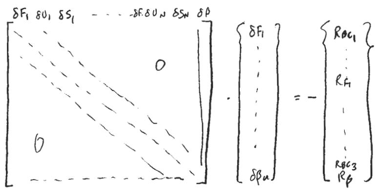
Note that the Jacobian has a sparse tridiagonal structure, except the row and column due to  $R_p$ . This can be handled by solving system in 2 steps.
