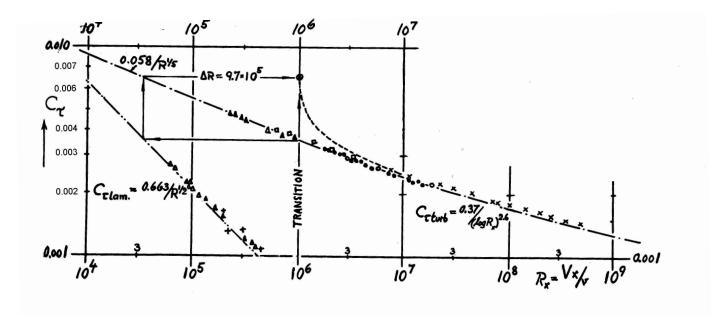
Figure 1: Skin friction coefficient,  $c_f$ , on a flat plate versus  $\text{Re}_x$  (from Hoerner [2]. Note:  $c_f$  is  $c_\tau$  in figure).
