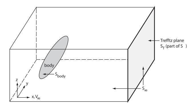
Upstream flow is  $V_{\infty}$  and is in x-direction. Thus, drag is the force in x-direction. Apply integral momentum in x to find induced drag.
