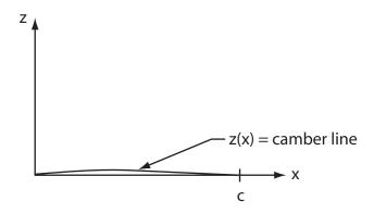
• Distribute vortices of strength  $\gamma(x)$  along chord line for  $0 \le x \le c$ .
