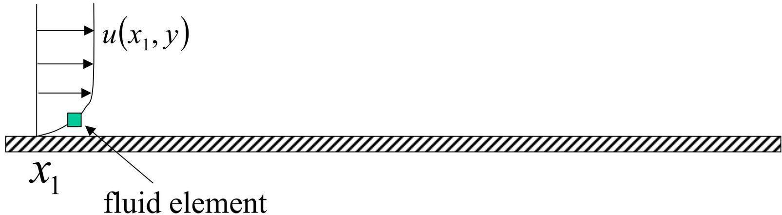
If the edge pressure is constant for the boundary layer sketched above, what is the direction of the net x-force acting on the fluid element:
