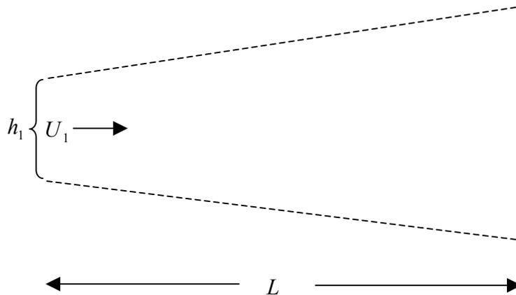
b) The diffuser is designed to decrease the velocity from  $u_e(0) = U_1$  to  $u_e(L) = \frac{1}{2}U_1$ . Assuming that the x-velocity (outside of the boundary layers) is independent of  $y$  and that the boundary layers are thin, determine the edge velocity as a function of  $x$ , i.e. find  $u_e(x)$  in the diffuser.
