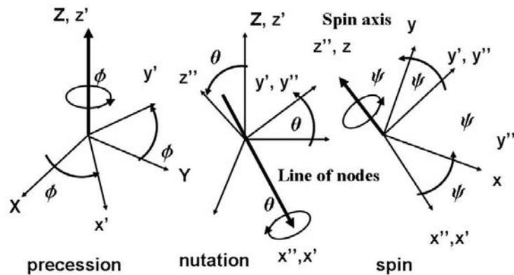
We first rotate from an initial  $X, Y, Z$  system into an  $x', y', z'$  system through a rotation  $\phi$  about the  $Z, z'$  axis. The angle  $\phi$  is called the angle of precession.
