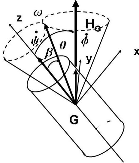
What we would see in this motion is a body spinning about the  $z$  axis with  $\dot{\psi}$  and "precessing" about the  $Z$  axis with  $\dot{\phi}$ —this is essentially a definition of precession. The  $\boldsymbol{\omega}$  vector, which is the instantaneous axis of rotation, is in the  $x, z$  plane.
