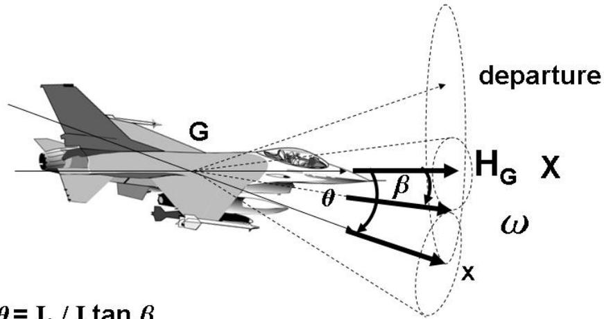
This could come as quite a surprise to a pilot. The question of what happens next is dependent upon the details of the aerodynamic forces, but just to comment on the historical record: in the first days of testing high-performance fighter aircraft, several test pilots lost control of their aircraft, in some cases with fatal results. This phenomenon, called roll coupling, is now well understood and incorporated into the design and testing of new fighter aircraft.
