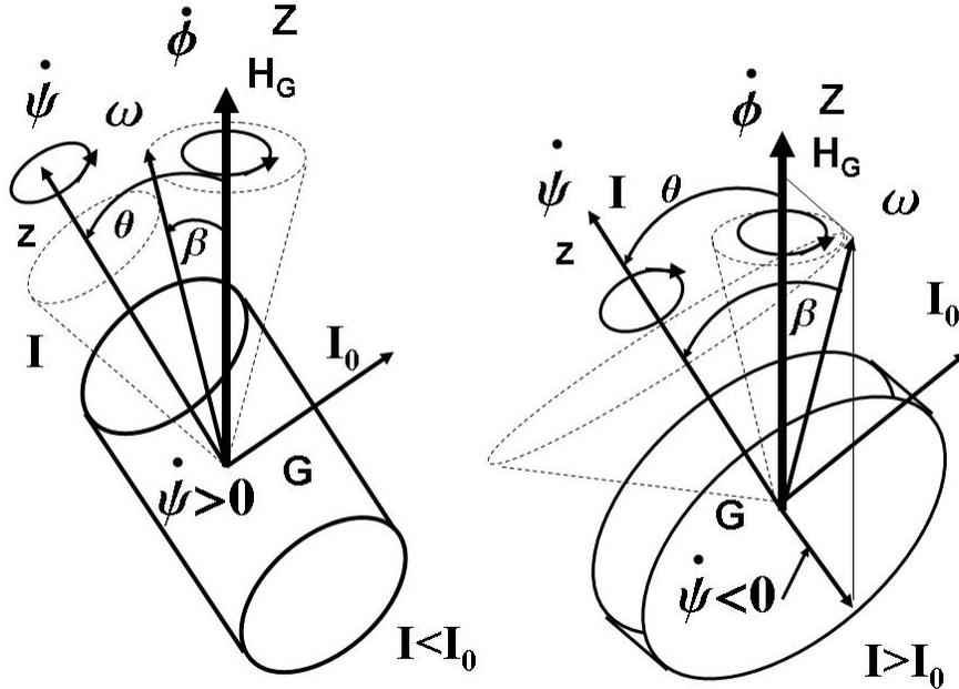
Two different solution geometries are shown: one for which  $I_0 > I$ ; one for which  $I_0 < I$ . Consider first the case where  $I < I_0$ . This would be true for a long thin body such as a spinning football, a reentering slender missile or an F-16 in roll.
