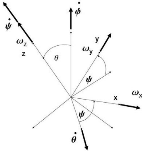
This is easily reorganized by taking the components of these angular velocities about the final  $x, y, z$  coordinate system using the Euler angles, giving
