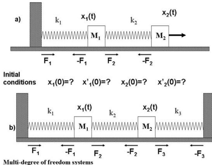
In this case, there are two independent variables,  $x_1(t)$  and  $x_2(t)$ ; their motion is not independent, but is coupled by their attachments to the springs  $k_1$ ,  $k_2$  and for system b),  $k_3$ . The sketch shows the forces  $F_i$  acting on the masses as a result of the extension of the spring; these of are equal and opposite at the ends of the springs. We consider both system a) and b). System b) is actually the simpler of the two systems because of its inherent symmetry.
