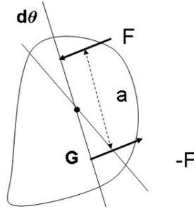
If  $M$  is constant, the work is simply  $W_{1-2} = M(\theta^2 - \theta^1)$ . In other words, the couples do work which results in the kinetic energy of rotation.
