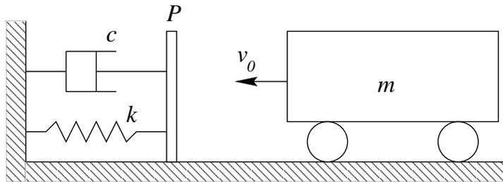
9. (9 points) The lightly damped system shown below is forced by an external force  $F = F_0 \sin \omega t$ . For two different values of the mass the motion  $x = X \sin \omega t$  looks as shown in A) and B). In which case is the mass  $m$  larger? Why?
