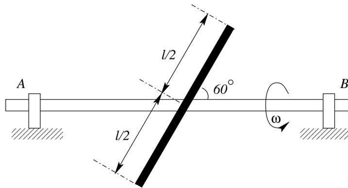
7. (9 points) A jet engine rotor has mass  $m$  and radius of gyration  $k_G$ . The center of gravity of the rotor is at distance  $l$  from the two supporting bearings. What are the **magnitudes** of the horizontal forces exerted by the two bearings on the rotor if the airplane is flying with velocity  $v$  along a horizontal circular trajectory with radius  $\rho$ . The dimensions of the airplane are small relative to the radius  $\rho$ .
