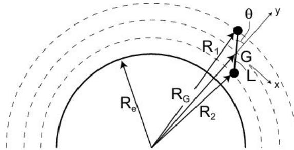
1. Recall that the gravitational force magnitude is  $F = gmR_e^2/R^2$ , where  $R$  is the local scalar radius to the center of the earth and  $R_e$  is the radius of the earth. However, the gravitational force is a vector pointing to the earth's center. Show that to account for both strength and direction of the gravity force at an arbitrary point, the vector representation is
