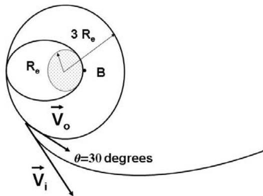
2-2a) Going backwards: determine the  $\Delta V$  necessary increase the velocity of the spacecraft from zero at the point  $B$  to the orbital speed of the Homan transfer orbit, ignoring the rotation of the earth and atmospheric drag.
