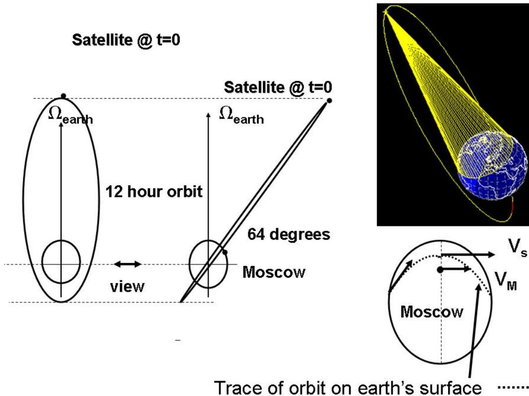
Determine the orbital parameters for a satellite with a 12 hour period. Ignore the rotation of the earth and the motion of the earth around the sun. In this case, the satellite will retrace its orbit twice per day. Two satellites will give reasonable coverage of the northern latitudes.
