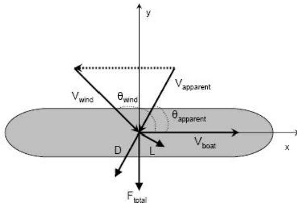
Figure 2: Top view of boat.
