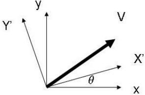
$$\begin{pmatrix} X' \\ Y' \end{pmatrix} = \begin{pmatrix} \cos \theta & \sin \theta \\ -\sin \theta & \cos \theta \end{pmatrix} \begin{pmatrix} x \\ y \end{pmatrix}$$
