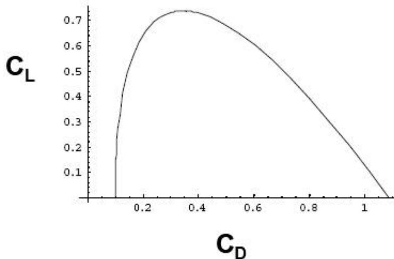
For this  $L/D$  and a wind speed of 20 knots, what is the maximum speed of the iceboat and what angle should the helmsman make to the true wind direction to achieve this speed? Does this angle have any significance relative to the plot of  $L/D$ ?
