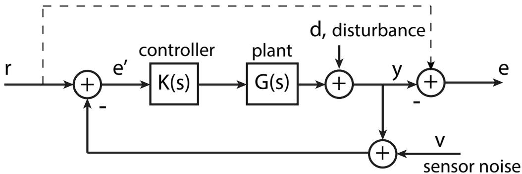
$e'$  is the error perceived by the control system;  $e$  is the actual error. The important transfer functions are
