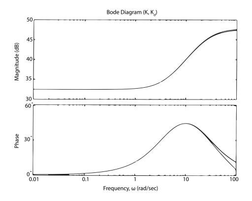
The phase lag in  $G_d$  is due to the effect of the zero order hold. To see why, consider sampling then holding a sinusoidal signal:
