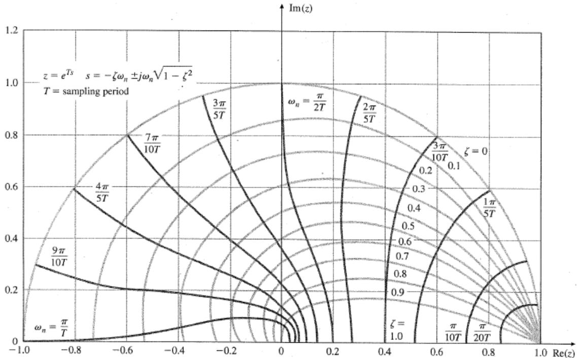
Figure 8.4 Natural frequency (solid color) and damping loci (light color) in the  $z$ -plane; the portion below the  $\text{Re}(z)$ -axis (not shown) is the mirror image of the upper half shown.
