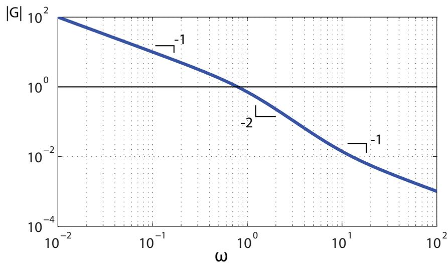
The slope at high frequency is  $-1$ , so it seems that we should be able to cross-over anywhere. However, in this case we need to look at the phase plot, since gain-phase theorem does not apply:
