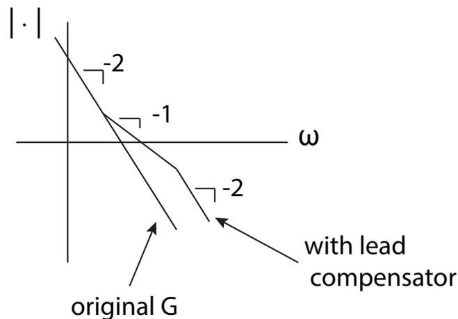
To get most phase lead for given lead ratio ( $b/a$ ), place pole and zero symmetrically around desired crossover. This maximizes average slope near crossover.
