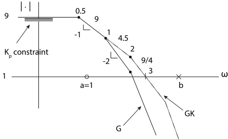
To get better slope at crossover, add lead compensator. It's *convenient* to place zero at  $s = -1$ , since this cancels plant pole, and makes Bode plot simpler. Working out the geometry, this puts the cross-over at
