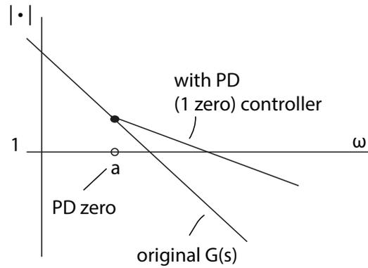
To get PD correct, need  $60^\circ$  phase lead from PD zero,
