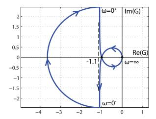
Note that arc at  $\infty$  is clockwise, because deformation at s=0 around pole is counterclockwise.
