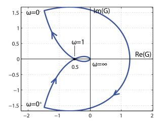
Note that deformation in contour (small semicircle in  $C_1$ ) maps to large semicircle in  $G(C_1)$ . Since there are no open loop poles inside  $C_1$ , the number of closed loop poles is
