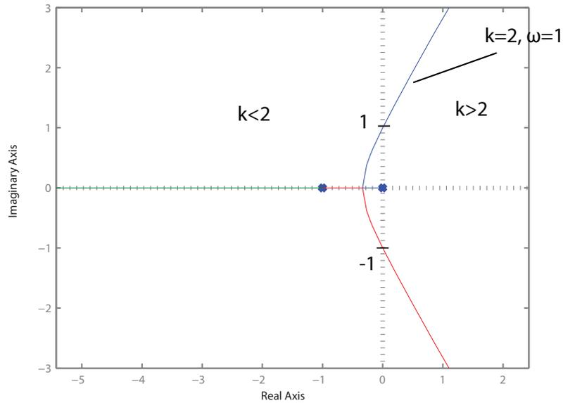
So neutral stability occurs for  $k = 2$ , corresponding to closed-loop poles at  $\omega = \pm 1$ . This result may be seen clearly on the Bode plot for this system.
