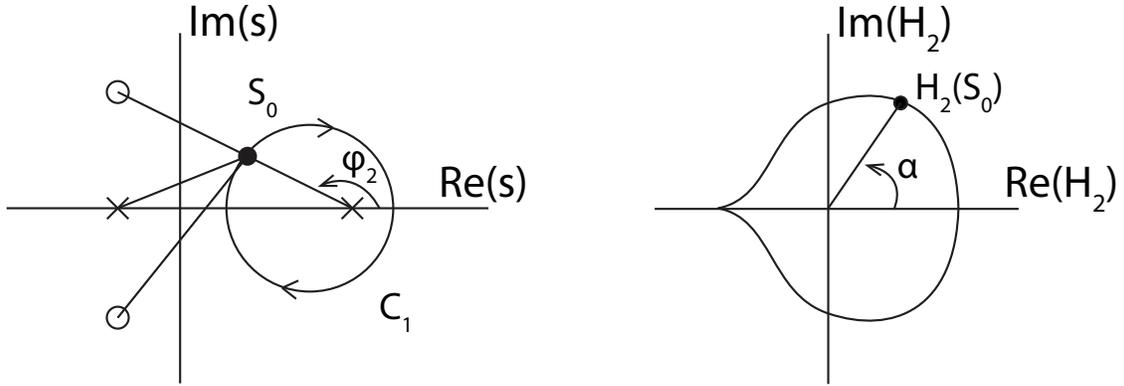
In this case, as we move once around  $C_1$ ,  $\Psi_i$ ,  $\Psi_2$ , and  $\phi_1$  return to their original values, but  $\phi_2$  decreases by a net  $360^\circ$ . As a result,  $\alpha = \angle H_2$  increases by a net  $360^\circ$ . But this is equivalent to saying that  $H_2(C_1)$  encircles the origin exactly once in a clockwise direction.
