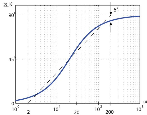
For  $K = \frac{1}{1+s/a}$ , the above magnitude and phase plots are flipped about  $|K| = 1$  or  $\angle K = 0^\circ$ .
