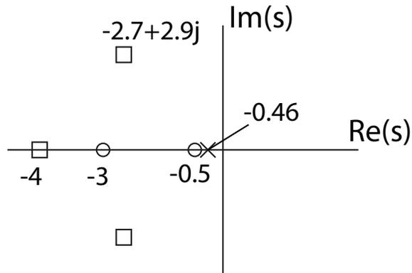
The near pole-zero cancellation of pole at  $-0.46$  means the effect of that pole is small, but it has a *very long time constant*. This pole is responsible for the small but long time constant error.
