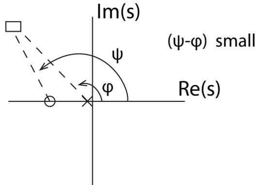
The change in phase angle at the desired pole location is small ( $\theta(5^\circ)$ ), so the locus (away from the origin) doesn't change much.
