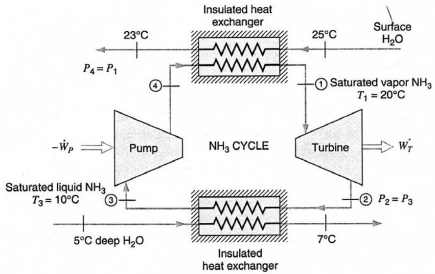
$$\eta_{s\text{Pump}} = 0.80; \eta_{s\text{Turbine}} = 0.80; \dot{m}_{\text{NH}_3} = 1000 \text{ kg/s}$$
