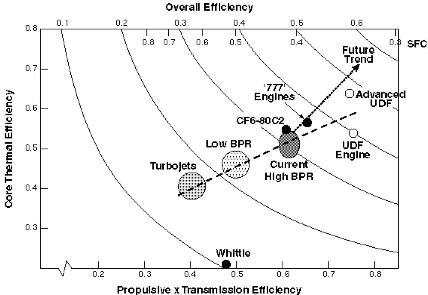
Trends in *thermal efficiency* are driven by increasing compression ratios and corresponding increases in turbine inlet temperature. Whereas trends in *propulsive efficiency* are due to generally higher bypass ratio engines
