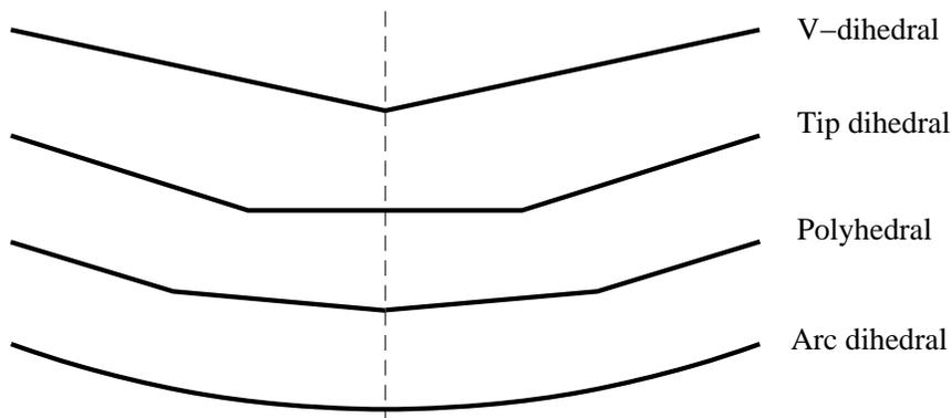
Figure 2: Different dihedral layouts approximating the ideal continuous arc dihedral distribution.
