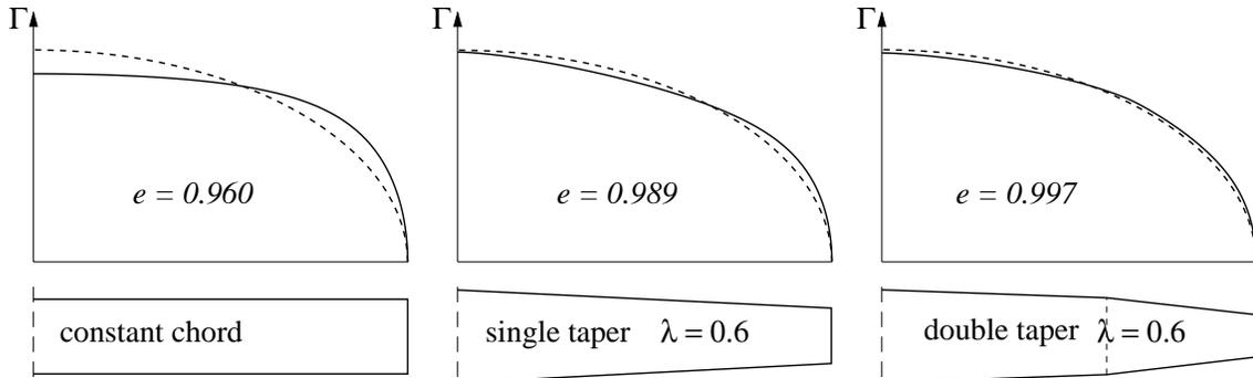
Figure 1: Span efficiency of three different planform untwisted wings. Dashed lines are elliptical loadings with the same lift.
