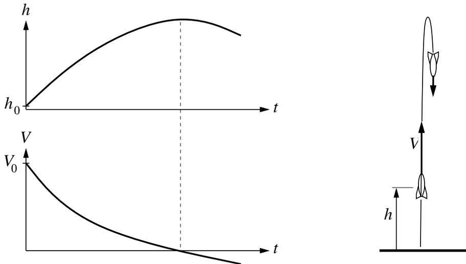
Figure 1: Time traces of altitude and velocity for a ballistic rocket trajectory.
