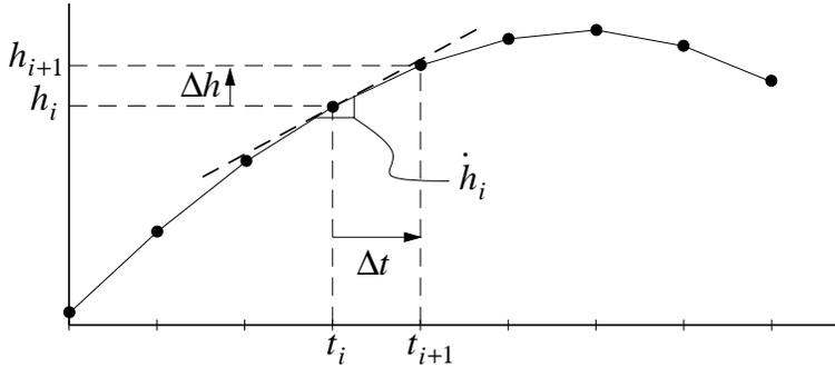
Figure 3: Time rate  $\dot{h}$  approximated with finite difference  $\Delta h/\Delta t$ .
