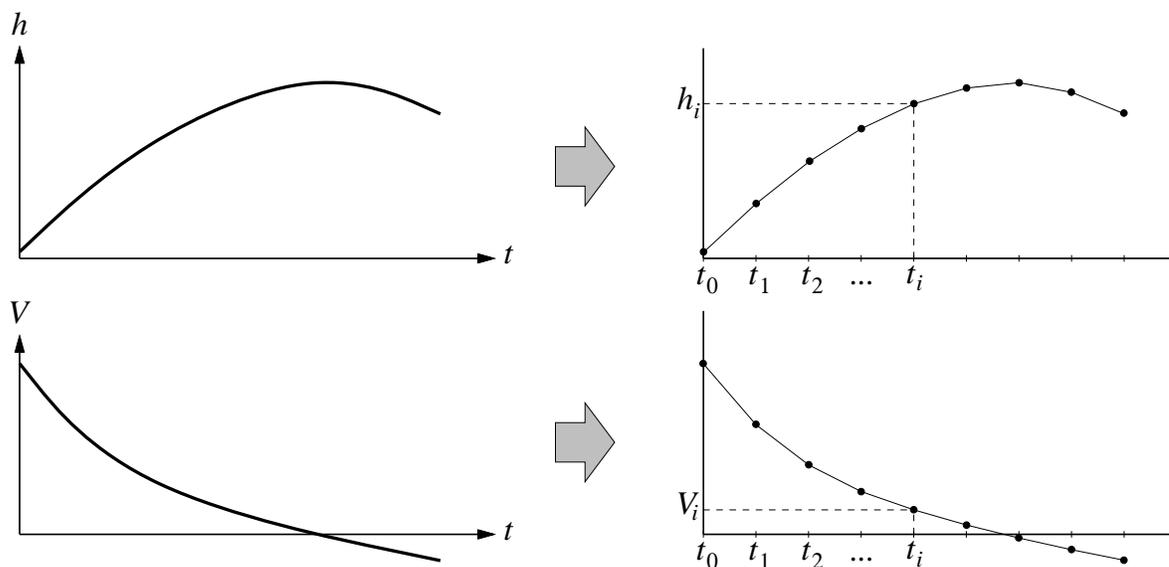
Figure 2: Continuous time traces approximated by discrete time traces.
