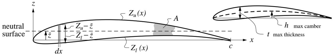
Figure 1: Quantities for determining and estimating the bending inertia of an airfoil section.
