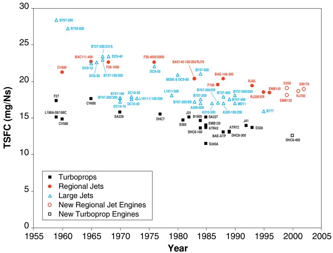
**Figure 1.9** Engine efficiency for commercial aircraft: specific fuel consumption (Babikian, R., *The Historical Fuel Efficiency Characteristics of Regional Aircraft From Technological, Operational, and Cost Perspectives*, SM Thesis, MIT, June 2001)
