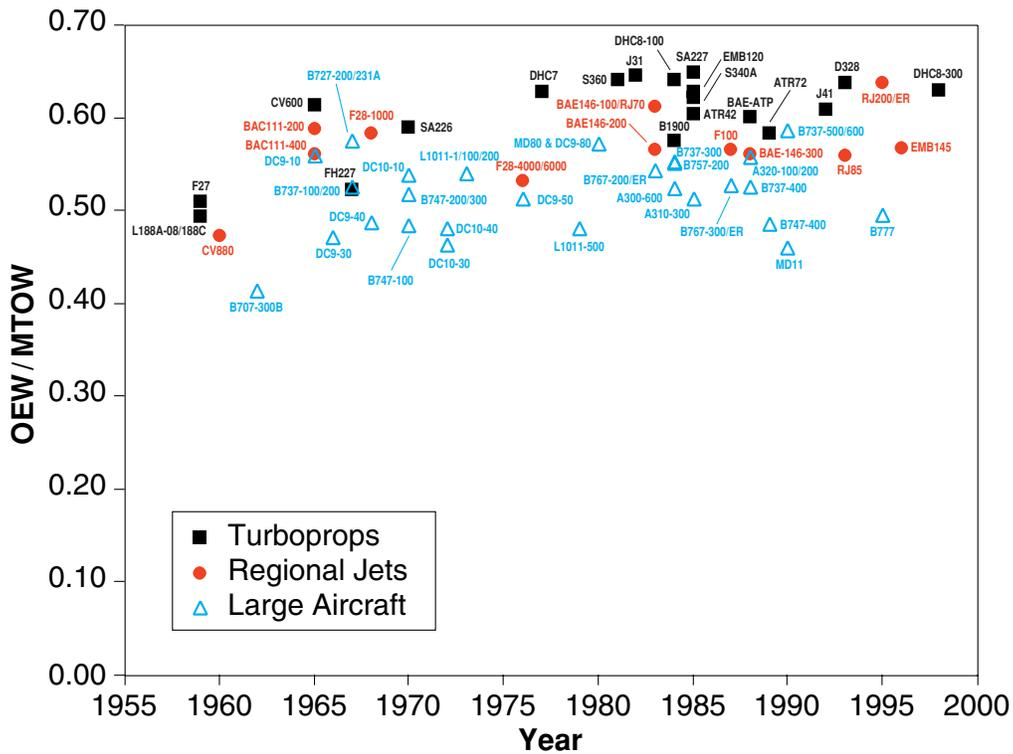
**Figure 1.6** Structural efficiency data for commercial aircraft: Operating empty weight over maximum take-off weight (Babikian, R., *The Historical Fuel Efficiency Characteristics of Regional Aircraft From Technological, Operational, and Cost Perspectives*, SM Thesis, MIT, June 2001)
