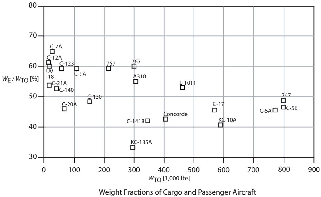
**Figure 1.5** Weight fractions for transport aircraft in terms of empty weight over max take-off weight (Mattingly, Heiser & Daley, *Aircraft Engine Design*, 1987)
