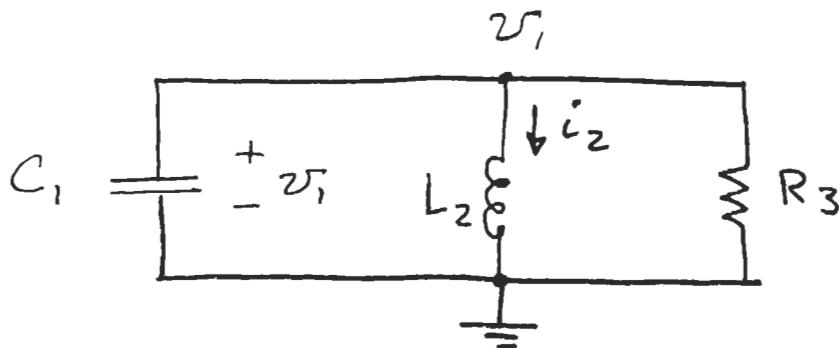
$$\begin{aligned} C_1 &= \frac{1}{2} F \\ L_2 &= \frac{1}{5} H \\ R_3 &= 1 \Omega \\ v_1(0) &= 1 V \\ i_2(0) &= 1 V \end{aligned}$$
