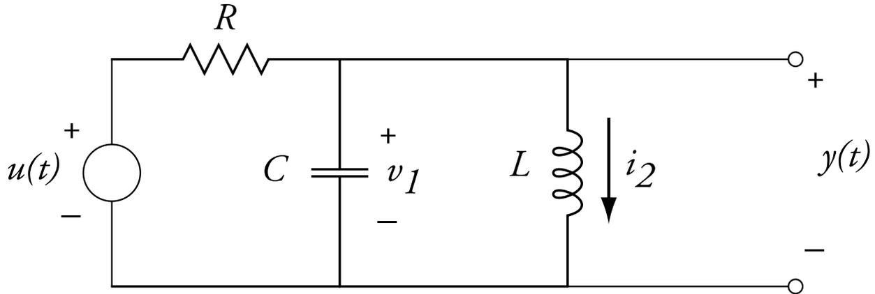
For the circuit above, take  $v_1$  and  $i_2$  to be the state variables. Find the differential equation for the state  $i_2$ .
