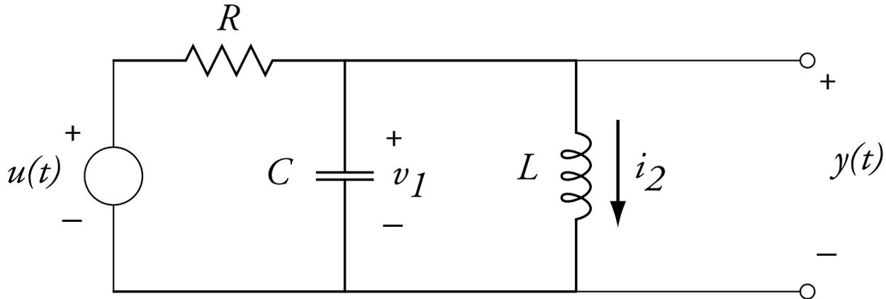
**For the circuit above, take  $v_1$  and  $i_2$  to be the state variables. The differential equation for the state  $i_2$  is**
