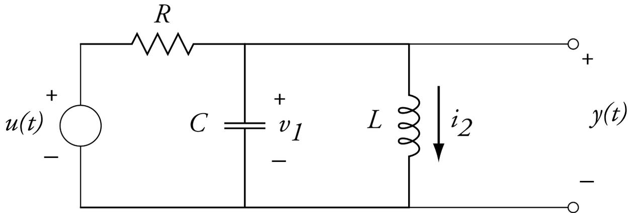
For the circuit above, take  $v_1$  and  $i_2$  to be the state variables. The differential equation for the state  $v_1$  is
