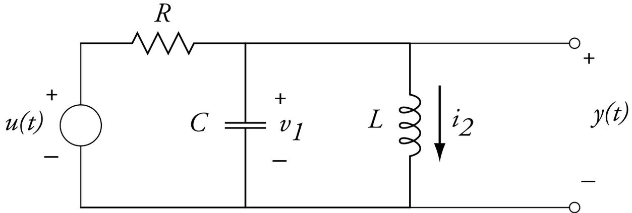
For the circuit above, take  $v_1$  and  $i_2$  to be the state variables. Find the differential equation for the state  $v_1$ .
